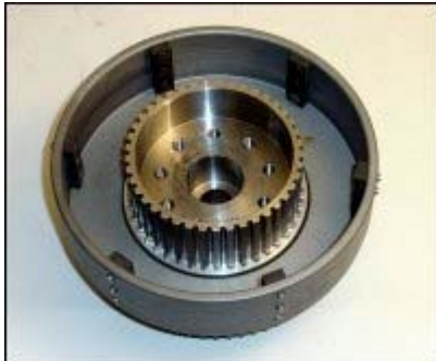
Hub installed in basket
