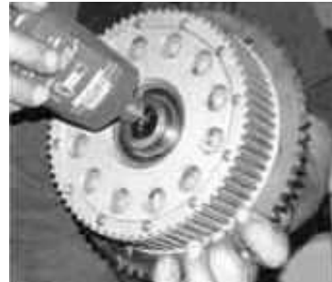
Fig. 8 Use Loctite® on spline hubs to ensure proper fit on mainshaft.
