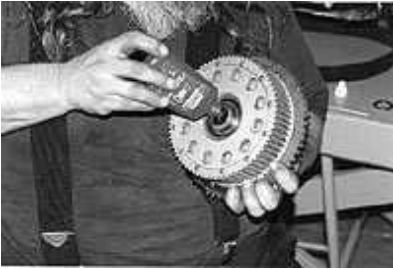
Fig. 5 Apply red Loctite® to spline hub before installing it onto mainshaft. This is for 1990-up models only.
