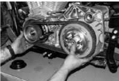
Fig. 6 Install both pulleys and belt at the same time.
