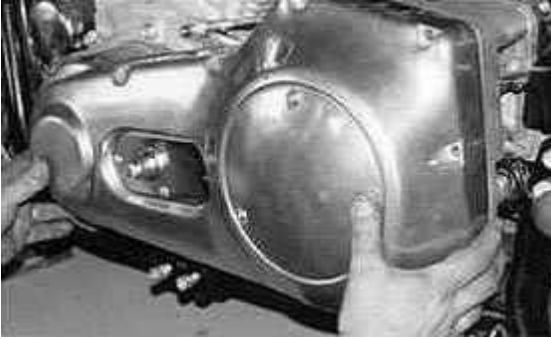
Fig. 12 Install outer primary cover with gasket
