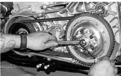
Fig.11 Install clutch adjusting rod supplied with kit 1986-up. and adjust clutch.
