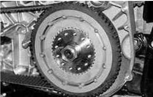
Fig. 9 Install sealed mainshaft nut supplied with 1990-up kits only. For 1986-89 you must use stock hub nut and the seal kit enclosed with kit. For Shovelhead you must use the stock hub nut with seal. Apply Loctite® to nut before installation.
