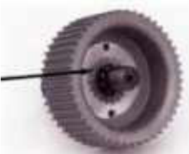
Fig. 7 If engine shaft spline protrudes as pictured, a washer is needed to compensate for protrusion of spline before washer and nut is installed.
