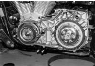
Fig. 1 Install pulleys and check for fit; some clearance may be necessary. Also check for alignment to determine if shimming may be necessary behind front pulley.
